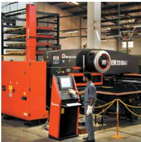
Hi-speed auto-loading CNC turret punch in action
