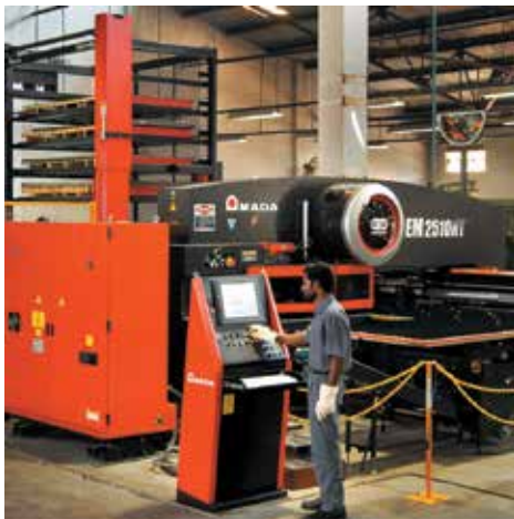
Hi-speed auto-loading CNC turret punch in action
